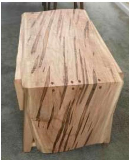
**Jake Herbst** used white ash to make this table with standard mortise and tenon legs and apron. Tabletop has an under-cut bevel that was done by hand.
